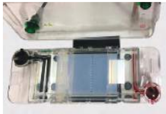
Fig 12.4: Agarose gel electrophoresis unit to separate nucleic acid
