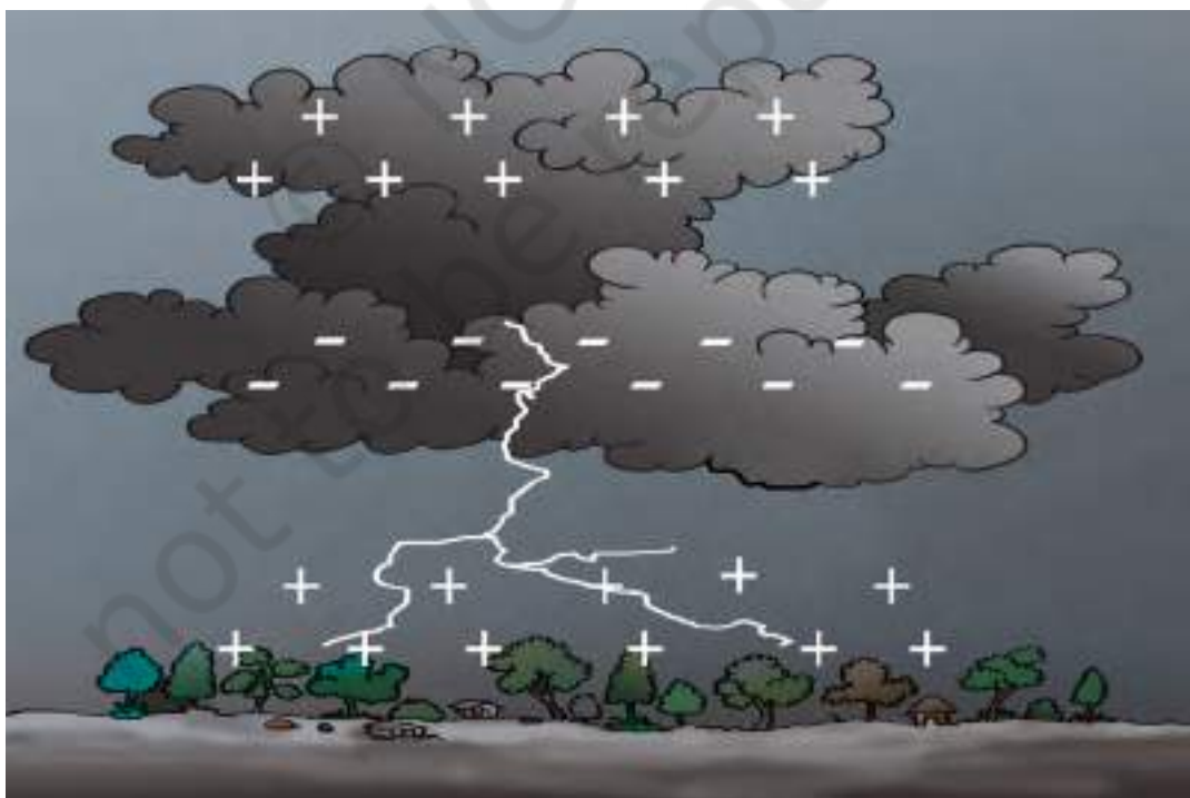
Fig. 12.5 : Accumulation of charges leading to lightning.
