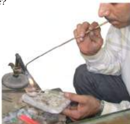
Fig. 4.14 : Goldsmith blowing through a metallic pipe
