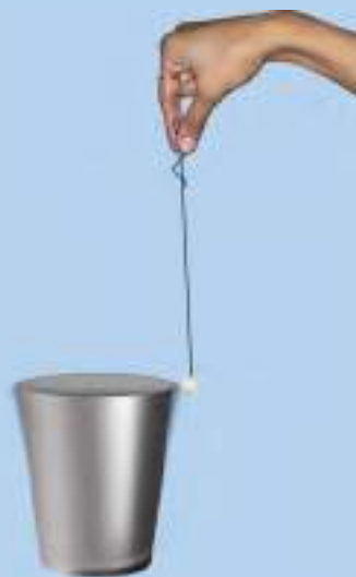
Fig. 10.17 : Thermocol ball touching the vibrating glass tumbler
